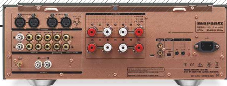
ABOVE: Two balanced (XLR) ins are joined by three single-ended line ins, one MM phono and a tape (recorder) loop on RCAs. The 4mm speaker binding posts offer A/B stereo and bi-amp operation. Wired remote supports system integration
