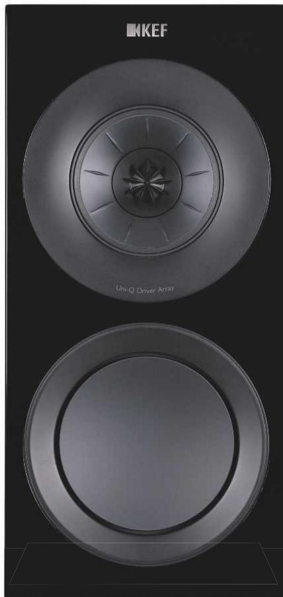
Constrained layer damping, originally conceived for the LS50, and a new approach to bracing, combine here to help 'dial out' the effect of the cabinet on the sound. Furthermore, the flexible port tubes are the result of computer modelling and extensive auditioning, and the crossovers are mounted on separate boards that are decoupled from the main cabinet structure to reduce vibration effects.
