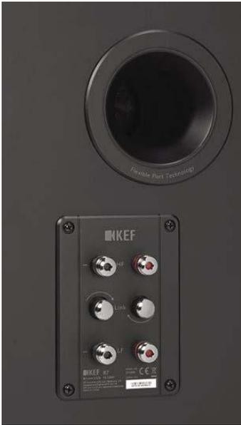
**The connection panel carries bass and mid/treble inputs for bi-wiring, but they are connected by a simple screw switch for mono-wiring.**
